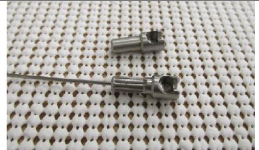
Part number: 30049-1 (X0091) 3 Series Standard Swivel: Specifications for crimping onto smaller core. Compatible with: .054, .062 core
