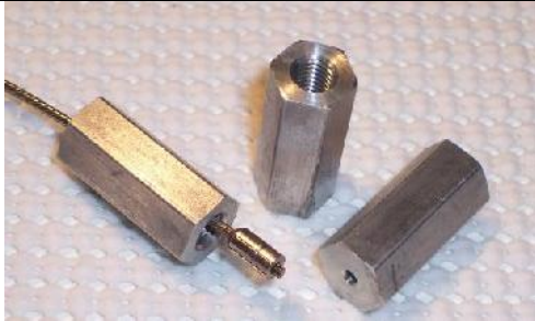
Part number: 82130500 (X1335-) Threaded Connector: Alum. ¼-28 x .5 I.D. s/w 98312400 Button on .062 strand. Compatible with: .054, .062 core
