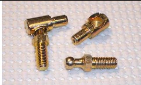
Parts: 82513000, Ball-joint (X1340-) with 10709, Ball stud (X1338-) Crimp-on Ball Joint w/retainer clip. Stud w/1/4-28 x ¾" thread: Plated Steel Compatible with: .054, .062, .075 core
