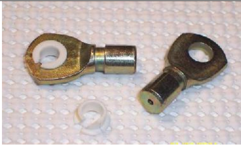
Parts: 30335-1, Term-eye (X1336-) with 10378, Bearing (X1337-) Groove to retain boot; ¼" ID w/bearing, 5/16" ID w/o bearing: Plated Steel Compatible with: .054, .062 core
