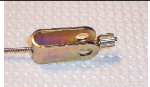
Part number: 30757-1 (X1334-) Clevis: Plated .256 Dia. cross hole shown with: 30245-1 Button on .062 strand. Compatible with: .054, .062, .075 core, can also use die cast barrel or ball.
